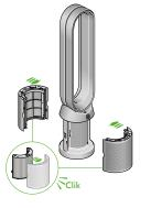
The air purifier fan with the filter covers open showing a HEPA plus carbon filter located in the filter covers. Arrows demonstrate that the filter covers will need to be assembled onto the base of the machine.
