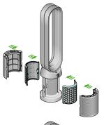
The air purifier fan with the filter covers open showing a HEPA filter located in the filter covers and a carbon filter. Arrows demonstrate that the carbon filter is fitted directly to the base of the machine and the filter covers will need to be assembled onto the base of the machine.
